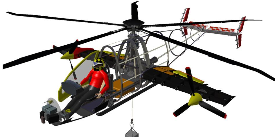
FIGURE 9.1: Cut away view of the internal components of the *Dart T690*.
