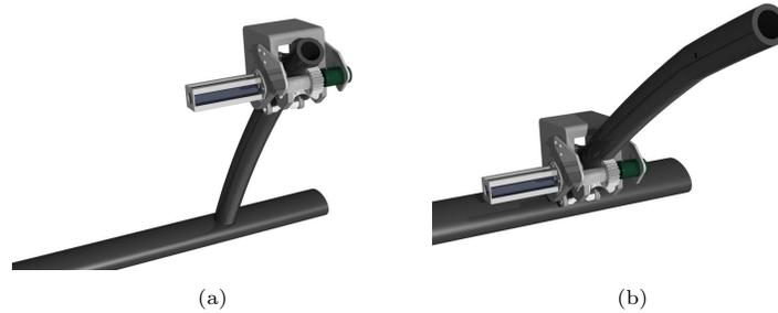
FIGURE 9.5: Landing gear (a) extended and (b) retracted.
