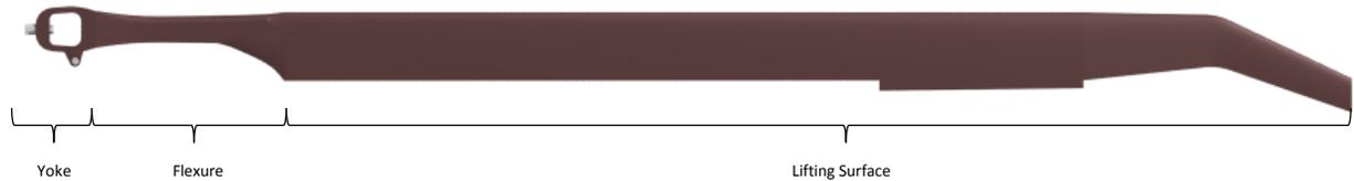
FIGURE 6.4: The three rotor blade structural sections.
