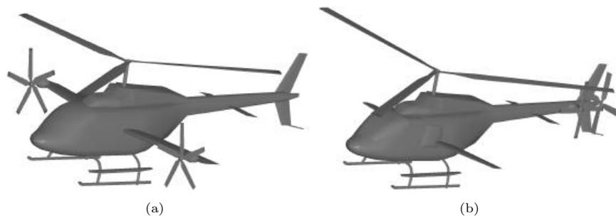
FIGURE 17.2: (a) Bell 206 with dual thrusters (b) Bell 206 with pusher propeller.
