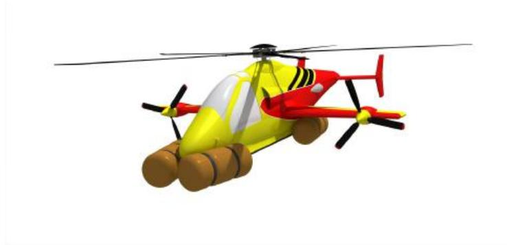
FIGURE 15.2: *Dart T690* with emergency flotation deployed, four floats are placed symmetrically around the c.g. for stability.
