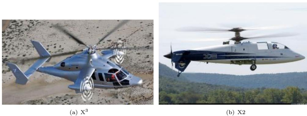
FIGURE 3.3: Eurocopter X<sup>3</sup> and Sikorsky X2 compound helicopters.
